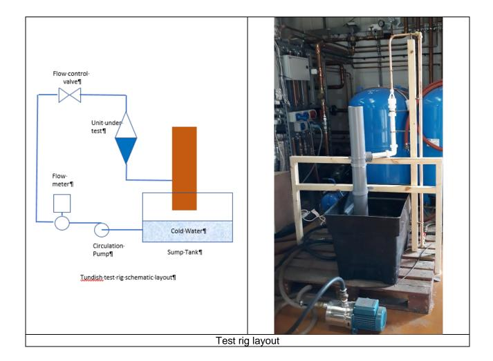
Each test was started at low flow and it was ensured that the lip and structs of the tundish were dry. The water pump was switched on with water flow set at zero or low flow and the flow was slowly increased stopping occasionally to photograph the state of the flow in the tundish. Notes were taken on the state of water in the tundish and any splashing or overflow occurring.
